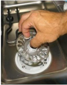
6. Clean the inner chamber of the tank.
