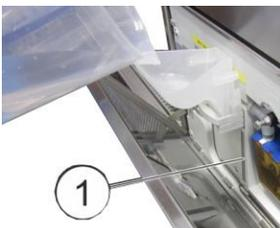
5. Use the funnel to help pour the chemical carefully into the machine until the storage container is full. Check the fill level via the fill level window (1).
