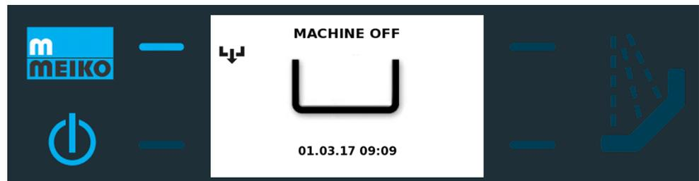
➔ Once the self-cleaning process is complete, the dishwashing machine will switch to **MACHINE OFF** mode.
