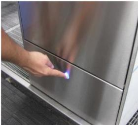
2. Press the illuminated blue button in the lower front panel.
